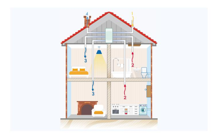
The diagram shows the Mechanical Ventilation Heat Recovery system. This is one of 3 types of ventilation we test and commission.
